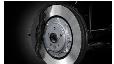
Opposed 6-piston brake caliper (front)
