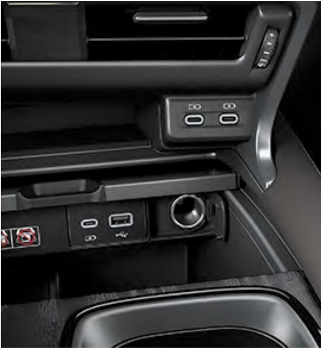
Center console: 3 USB Type C charging and USB Type A multimedia communication ports, DC12V
